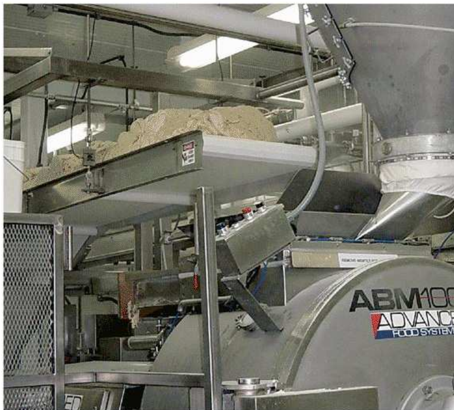
Donatos Pizzeria uses a mixer that automatically collects scrap on a conveyor and feeds it into the hopper.
