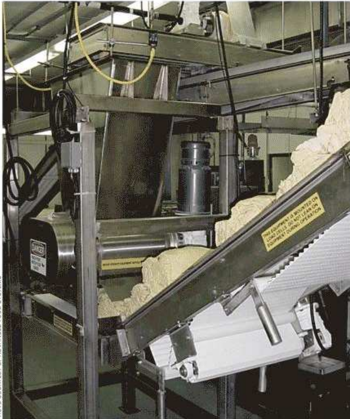
In continuous mixing, ingredients are fed into the mixer nonstop and dough continuously feeds out.
